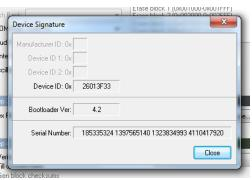
If the communication is working it is possible to proceed with the firmware update. Click on "close" on the "Device Signature" window. In the Flash Magic main window, click on "Start" to begin the programming. Wait until the end of the process, then turn off and on the FDM-DUOr.
