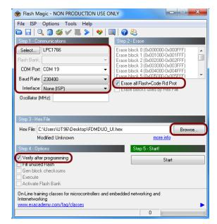
Check the communication with the FDM-DUOr clicking on "ISP" and then on "Read Device Signature". If the communication with the FDM-DUOr is working, a new window with some device information is opened.
